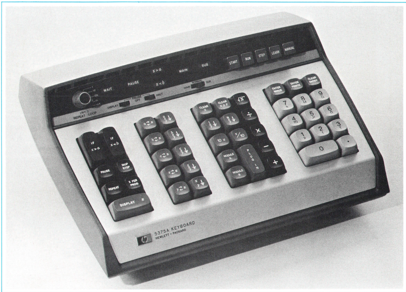
Fig. 1. Model 5375A Keyboard is an external programmer for Model 5360A Computing Counter. Programs can be executed manually, or learned and executed repetitively. The Keyboard can make comparisons, do program looping and branching, and insert constants into programs.
